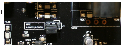
MPX Loopthrough Jumper in off position
